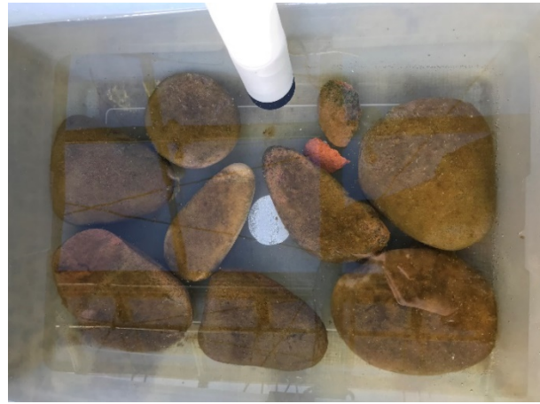
Figure 9. Artificial stream experiment at the Rocky Mountain Research Station in Flagstaff. 1) Experimental setup with recirculating tank, baskets of cobble with mudsnails (control, small, large snails), and gpp tiles; 2) Whole-tank gpp experiment with cobble from each basket, incubated for 18+ hours in water bath, with continuous reading O_2 mini-dot sensor; 3) Cobble with mudsnails; and 4) Algal growth after five months in artificial stream (June-November 2019).
