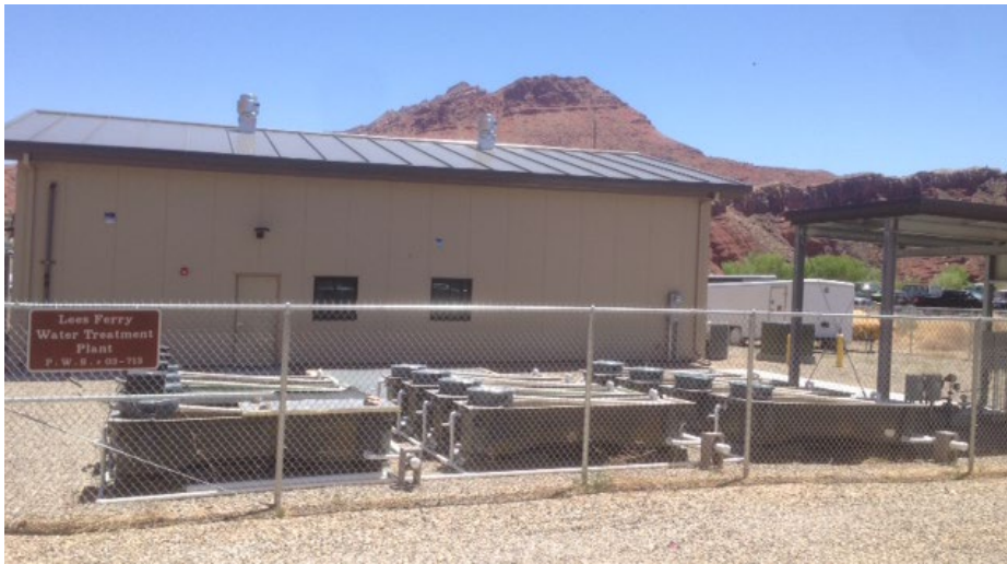
Figure E.2.3a. Artificial stream experiment tank configuration adjacent to the National Park Service Water Treatment Plant in Lees Ferry. Untreated water is drawn from underground pipes coming from the Colorado River ~200 meters away.
