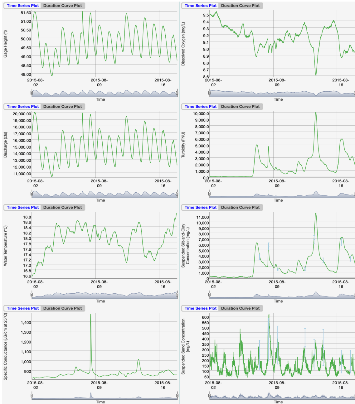
Figure 3. Plots of 15-minute gage height (i.e., stage, water elevation), water discharge, water temperature, specific conductance, turbidity, dissolved oxygen, suspended-silt-and-clay concentration, and suspended-sand concentration for the two-week period 8-2-2015 through 8-16-2015 at the Colorado River above Diamond Creek gaging station. Light blue dots with 95%-confidence-level error bars indicate episodically measured silt and clay concentrations and sand concentrations (from physical suspended-sediment samples) used to verify the two-frequency acoustical suspended-sediment measurements. Variability in each of these parameters over this two-week period arises from the interaction of dam operations with tributary floods. Plots from Project A’s website at https://www.gcmrc.gov/discharge_qw_sediment/ (U.S. Geological Survey, 2024).
