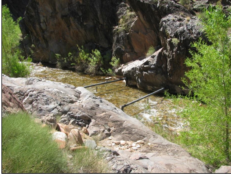
Figure 2. Remote full duplexing PIT tag antennas in Shinumo Creek. Antenna 1 (right) is upstream of 2.
