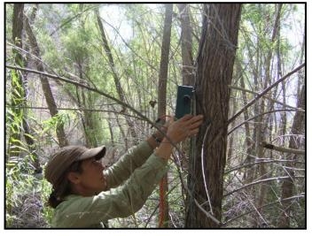
**Figure 4.** Securing a Song Meter SM2 Platform sound recorder onto a willow tree, river mile 275, river right, Grand Canyon, Arizona.
