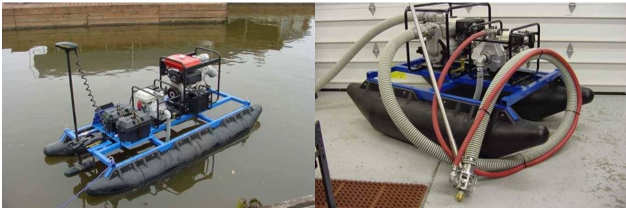
FIGURE 7 Examples of Small Raft Mounted Hydraulic Dredge Systems.
