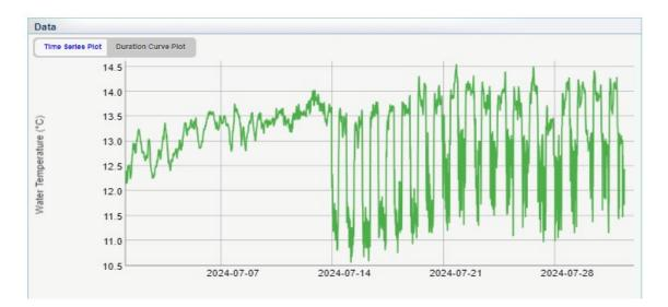
Below GCD. Max temperatures are a good indicator of normal penstock release temperatures, low temperatures include cold bypass releases. No updates since 8/1 - poor mixing, not very reliable for overall river temp
