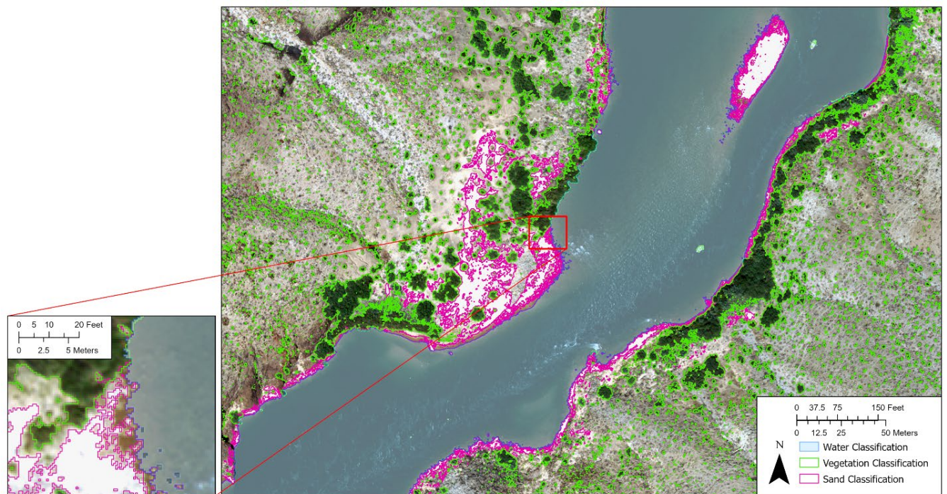
Figure 2. Example landcover classifications of the low-flow river channel at 8,000 ft 3 /s (water classification); total riparian vegetation (vegetation classification), and sand and other river sediment deposits (sand classification). For each overflight image dataset, GCMRC publishes USGS data releases of these most basic, fundamental maps of landcover covering the entire river corridor from Glen Canyon Dam to Lake Mead at Pearce Ferry. Various GCMRC projects leverage the landcover classifications, with imagery and topographic data for science that relates observations of environmental change in the Colorado River ecosystem to dam operations, other land use and management activities, climate, and other factors.
