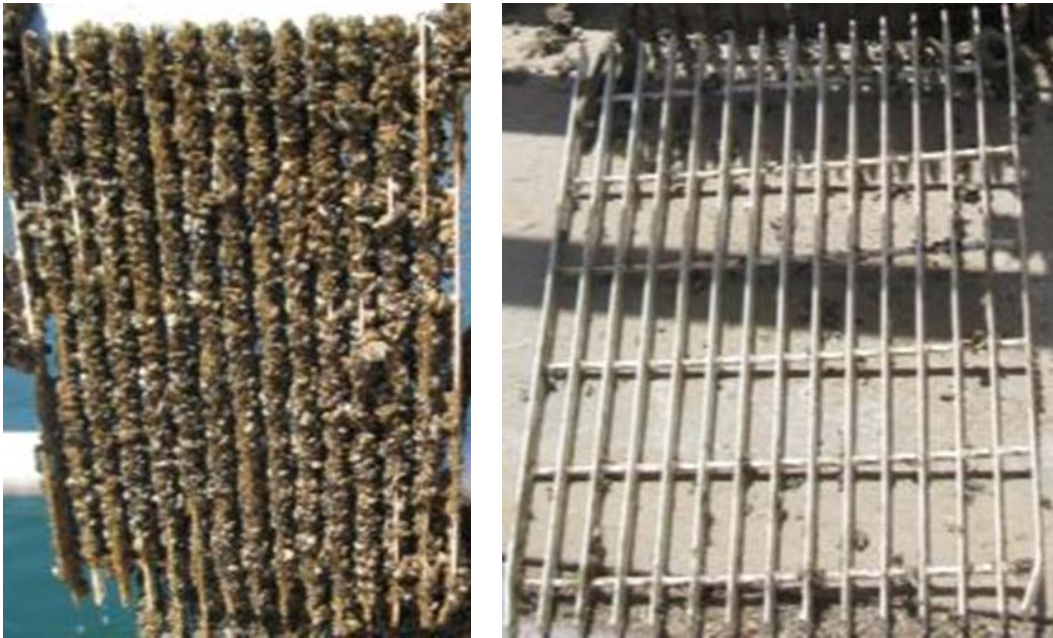
Figure 12. Grate treated with RTV Silicone ice phobic coating, before cleaning (left) and after cleaning (right), May 2014.
