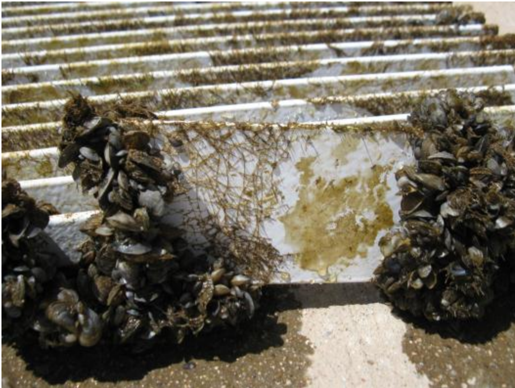
Figure 6. Silicone oil-free version of Silicone FR #1 after 22 months of exposure.
