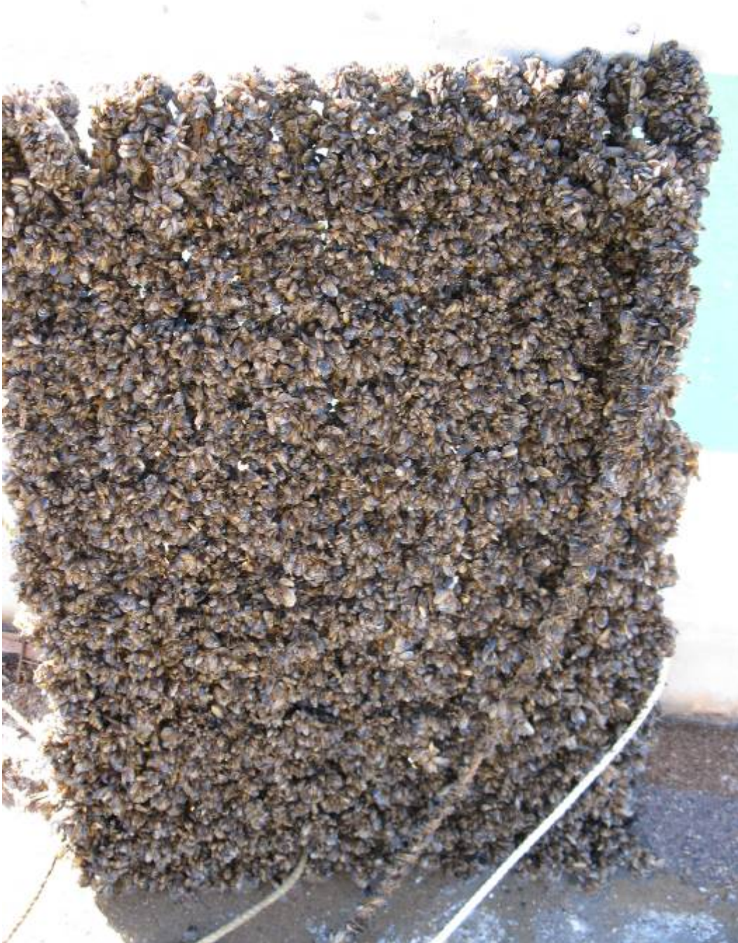
Figure 4. Uncoated steel after 7 months of exposure in dynamic conditions. Test period May 2008 to December 2008.
