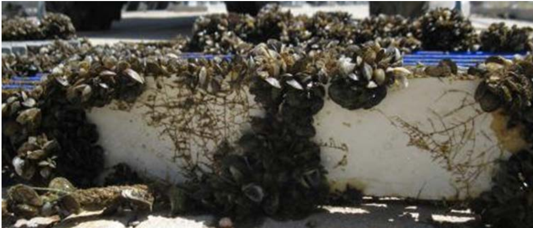
Figure 9. Panels coated with experimental formulations from 2012-MTA-8-1003 #1 and #2, exposure at 18 months.
