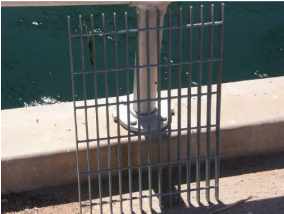
Figure 3. Coated floor grate before being hung from the forebay trashrack structure at Parker Dam.
